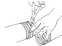
At last cut cleanly the hose material along the reinforce-spiral.
